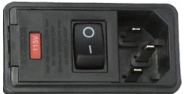
Connect power to the rear of the server. For servers with an IEC inlet, turn the switch from '0' to '1'. If possible leave the power on at the rear of the server permanently, as this keeps the key capacitors powered and so ensures the server is always ready to perform at its optimum audio quality. You may even prefer to leave the server booted up permanently for the best sound.
